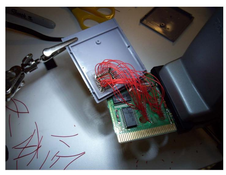
If you pre TIN your wire leads in the same manner, this will greatly improve your soldering work. Just be careful not to get to close to the adjacent contacts, a solder blob can be a pain to remove, especially if you run out of Flux and Copper wire wick.
